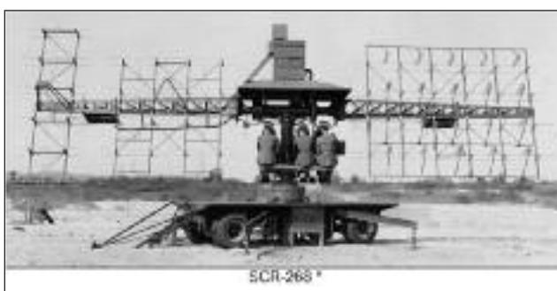
Figure 2: Exposed operators sat on a SCR 268 (NB this photograph is not of 105 Radar Station) (www.vectorsite.net).
